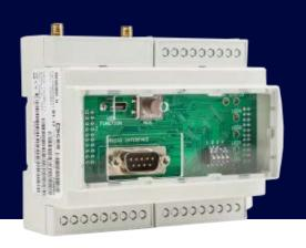
**REWIND** is a communication interface gateway through GSM / GPRS / LTE for a customer asset such as, a generator, light tower, fuel tank, etc... For the automatic data transmission to the SMARTCLOUD remote monitoring and control solution.
