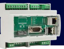
**DANCE** is an electronic device aimed for the monitoring of the status, parameters and operations of a genset, tower light, or a fuel tank, etc... via ETHERNET TCP/IP.
