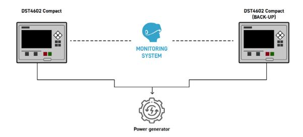
In sensitive contests, it is necessary to ensure a safe control of the genset.
