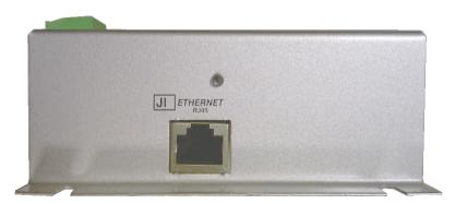
The CanBridge uses the Ethernet line to send data and receive commands using IEC 60870-5-104 protocol (see paragraph "4.5 Application E - Gateway IEC60870-5-104").
