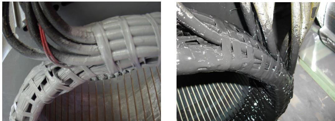
Grey treatment (marinization) on the left, TOTAL+ treatment shown on the right. The EG43 grey varnish, is an high temperature insulating enamel that forms a tough and flexible film, with excellent moisture and chemical protection. It is water and oil proof, and also protects windings from abrasion. It is applied spraying an over coating layer over the impregnated winding, or dipping the stator in a varnish barrel for superior treatments
